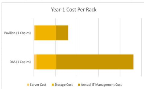
The "DAS" configuration consisted of 16 2U servers, each with 2x6.4TByte SSDs. The above YCSB test demonstrated that using Pavilion allows us to reduce the number of servers. Eliminating direct-attached SSDs allows us to use 1U servers, saving a large amount of acquisition costs, rack space and power and cooling. Through the use of thin provisioning and space-efficient snapshots, the total capacity can be reduced for the same usable capacity.
